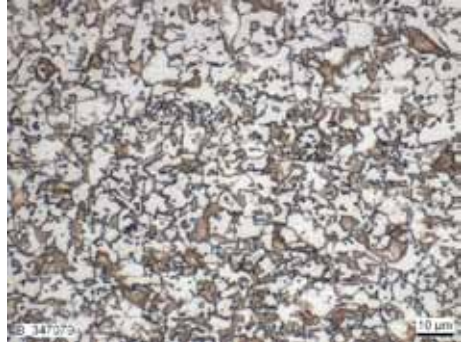
Fig. 1: Microstructures of two steels with different C and Mn contents after intercritical annealing.
